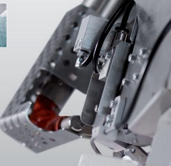
Upgrade of the market leader! Hot-air taping machine from PFAFF INDUSTRIAL for welding continuous seams on water-resistant, waterproof and breathable materials with new technical features:
